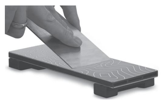
• Keep the bevel of the chisel/plane iron flat on the stone.
