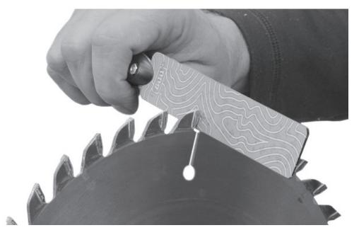
Keep the diamond surface flat to the face of saw tooth.
